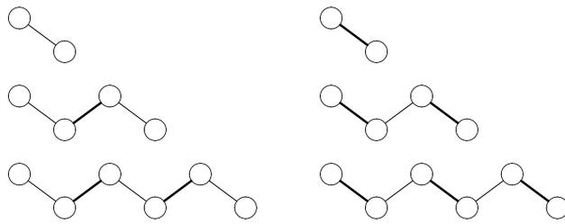
**Fig. 5** Augmenting paths (at left) and the effect of applying them (at right). The first augmenting path carries out a simple assignment; the second carries out two assignments and one deassignment; and so on. In each case the size of the matching increases by one. No matching edge may initially touch the first or last node.
