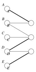
Both are maximum, since all three supply nodes are matched in each; but the competitors of C in the first matching are A and B, while the competitors of C in the second are D and E.
