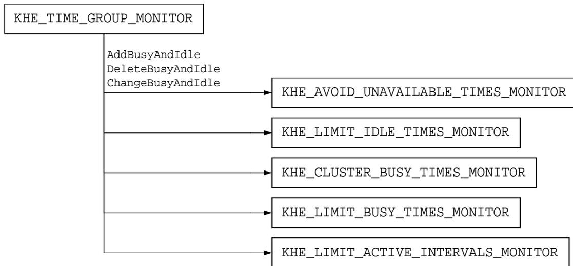
When a monitor is attached, function `AddBusyAndIdle` is called instead, and when a monitor is detached, function `DeleteBusyAndIdle` is called instead.
