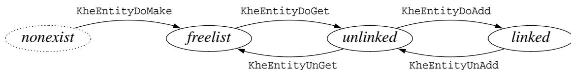
State *nonexistent* means that the object does not exist; *freelist* means that it exists on a free list; *unlinked* means that it exists, not on a free list, not linked to the solution, but referenced from somewhere on some path; and *linked* means that it exists and is linked to the solution.
