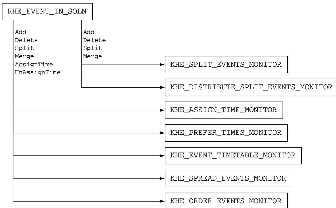
Split events and distribute split events monitors do not need to know about time assignment and unassignment. Based on the calls they receive, they keep track of meet durations and report cost accordingly. Assign time and prefer times monitors are even simpler; they report cost depending on whether the meets reported to them are assigned times or not.
