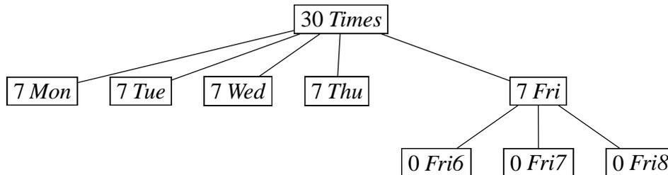
A postorder traversal of this tree may be used to deduce that workload demand nodes for  $r$  are needed for one *Mon* time, one *Tue* time, one *Wed* time, one *Thu* time, one *Fri6* time, one *Fri7* time, one *Fri8* time, and three arbitrary times. In general, each tree node contributes a number of demand nodes equal to the size of its set of times minus its number minus the number of demand nodes contributed by its descendants, or none if this number is negative.
