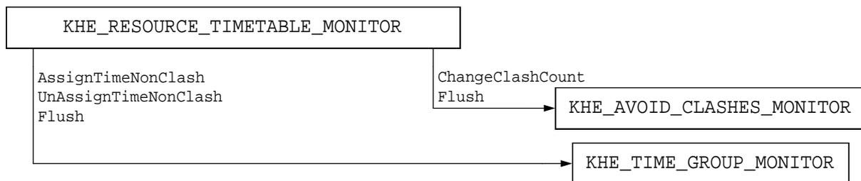
An avoid clashes monitor is notified whenever the number of meets at any one time increases to more than 1 or decreases from more than 1 (operation `ChangeClashCount` above). It uses these notifications to maintain its deviation. It updates the solution when a `Flush` is received from the timetable at the end of the operation.
