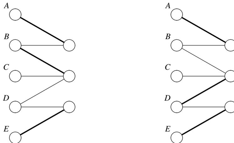
Both are maximum, since all three supply nodes are matched in each; but the competitors of *C* in the first matching are *A* and *B*, while the competitors of *C* in the second are *D* and *E*.
