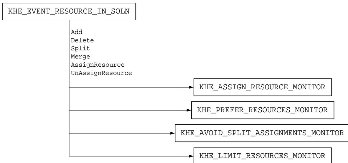
None of these monitors cares about time assignments and unassignments. Assign resource monitors and prefer resources monitors are very simple, reporting cost depending on whether the tasks passed to them are assigned or not.
