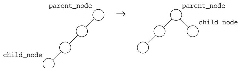
In each case where a complete chain of assignments reaches from a meet `meet` of `child_node` to a meet of `parent_node`, `meet` will be assigned afterwards, to the meet at the end of the chain, with offset equal to the sum of the offsets along the chain. This is valid (it does not change the timetable). Where there is no complete chain, `meet` will be unassigned afterwards.
